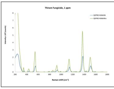
The sensitivity improvement with QE Pro-Raman+ is evident in these measurements of the fungicide thiram. The use of SERS nanoparticles also contributes to system sensitivity.
